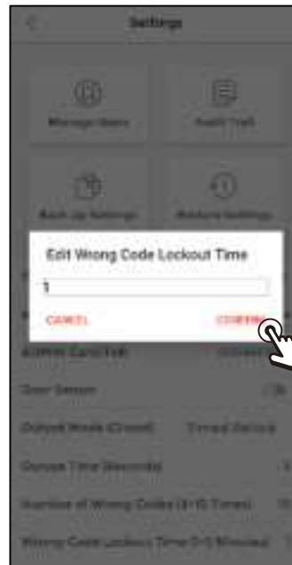
Enter the desired time (1~5 minutes) for the device to lockout and click Confirm
