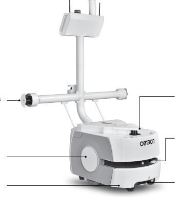
Latch System Automatically engages and disengages with cart units.
