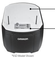
AUX Power & I/O Internal connections to power and control custom topper models.
