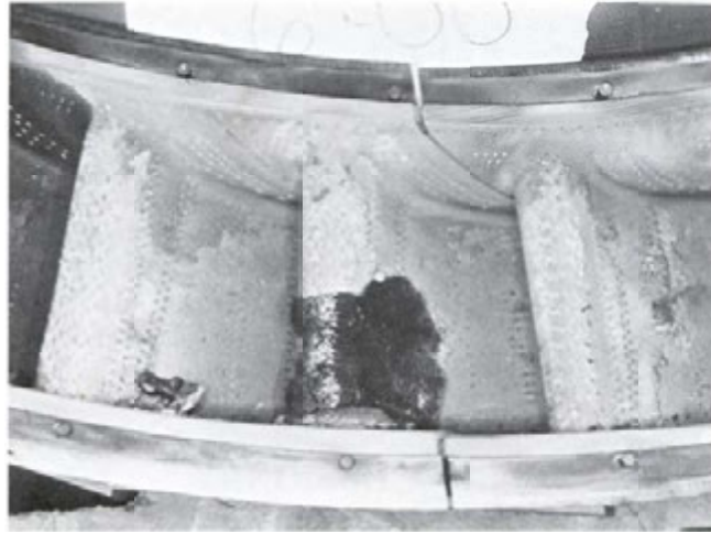
Figure I-4-1 a). Dark, glassy deposits of remelted volcanic ash on leading edge of stage-1 high-pressure-turbine nozzle guide vane. (from Przedpelski and Casadevall)
