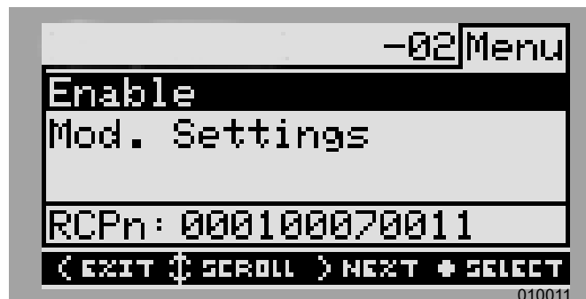
Figure 6-7. Enabling Inverter (2 of 4)
