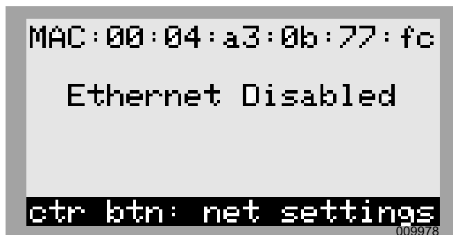
Figure 6-24. Ethernet Configuration (1 of 4)
