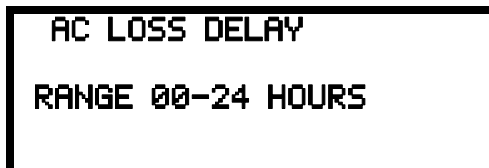
AC Loss Delay Screen #1
