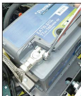
Fig. 10-1 Loosening the terminals
