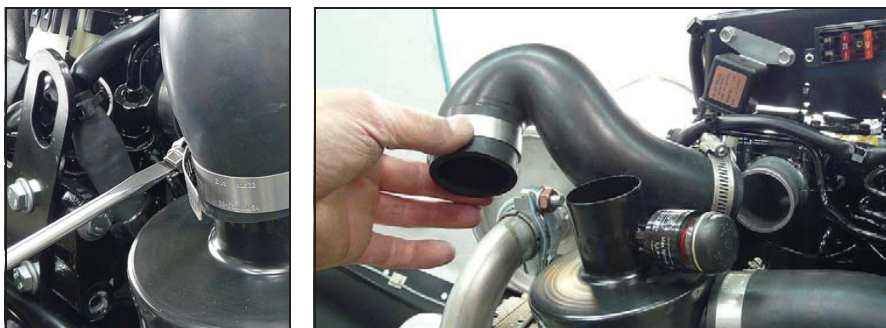
Fig. 10-11 Remove the air filter hose at the top
