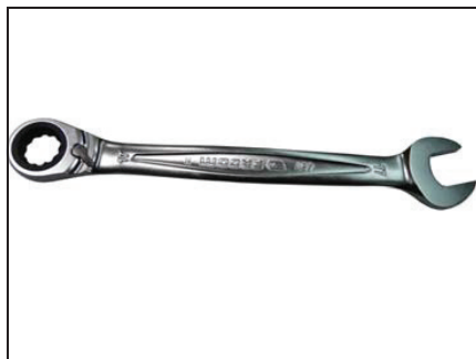
Fig. 10-17 Box-end ratchet wrench/Rotate crankshaft
