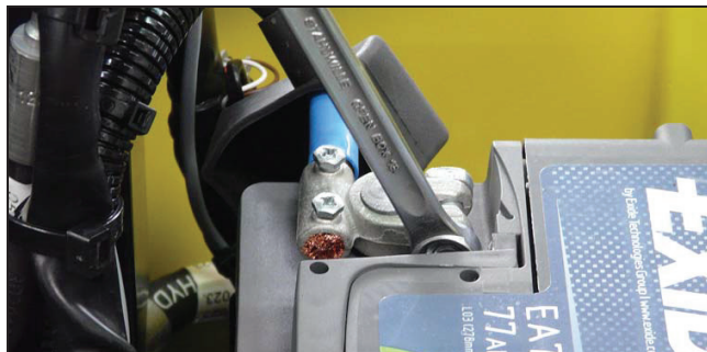
Fig. 10-9 Disconnect the battery
