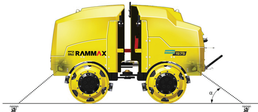
Fig. 12-3 Lashing the roller/side view
