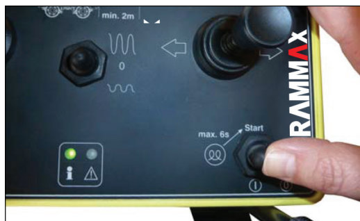
Fig. 7-2 Start the engine/Infrared sensor
