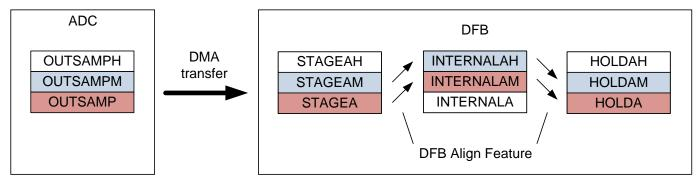
The ADC is MSB aligned to OUTSAMPM, whereas the DFB is aligned to its MSB. i.e., STAGEAH. In this scenario, the DFB will not recognize that a valid data has been placed in its
