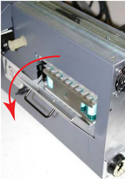
Analyzer Filter Door
