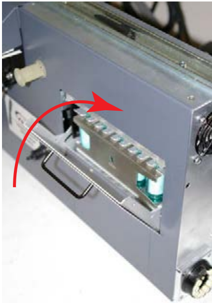
Analyzer Filter Door
