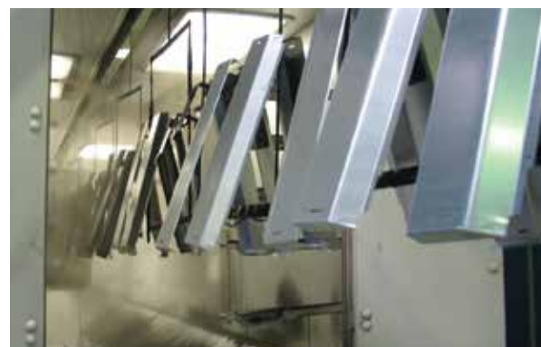
Alkaline cleaner being sprayed on parts.
