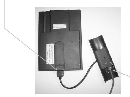
**2.** Plug in the Ethernet cable in the Travel hub. Insert the Ethernet connector into your Travel hub.
