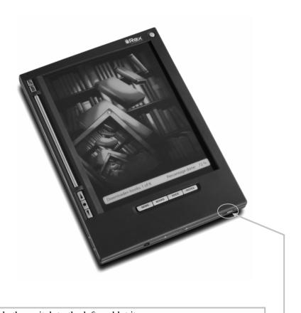
**1.** Slide the switch to the left and let it go. Besides from shutting the device off, the keys are also locked and the display is blanked.
