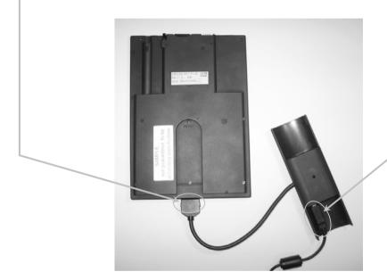
**3.** Insert the other end of the USB Cable in to your PC. NOTE: The USB port on the top of the device only accepts USB sticks. It is NOT meant for a USB cable.
