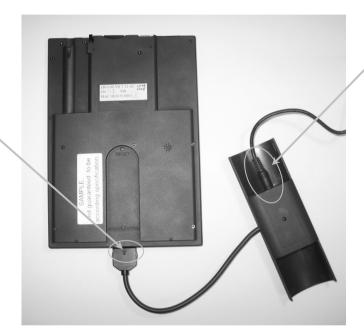
The battery of your iLiad is fully charged when the red LED stops burning. A complete empty battery takes up to two hours to be fully charged.
