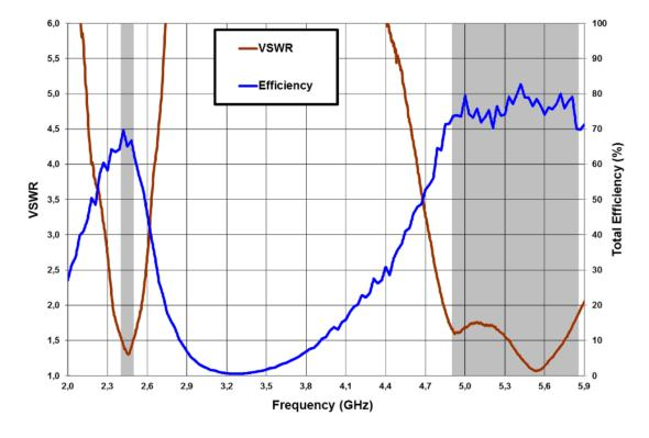
VSWR (Voltage Standing Wave Ratio) and Total Efficiency versus Frequency (GHz).
