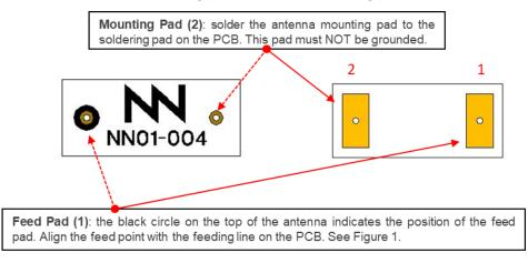
Figure 6 – Pads of the Compact Dual-band Reach Xtend<sup>™</sup> chip antenna.
