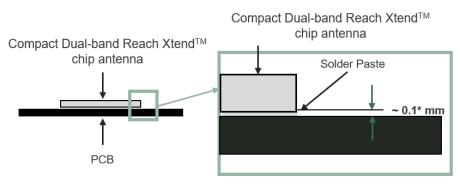
Figure 7 – Soldering Details.
