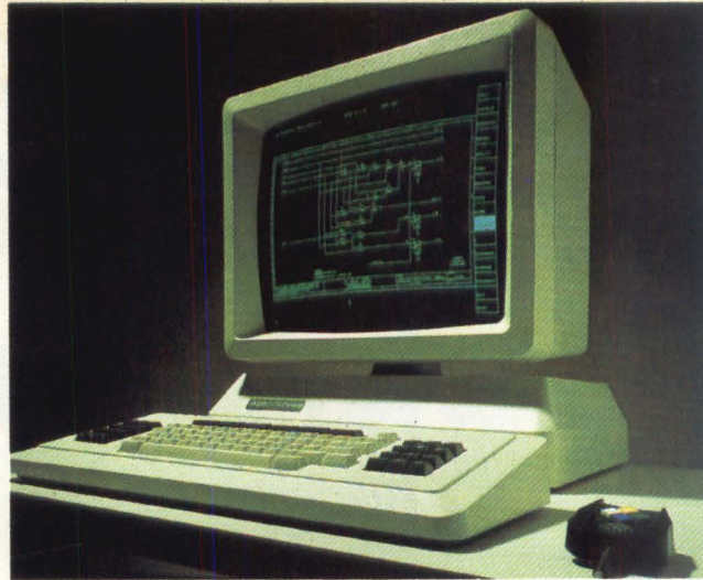
Figure 2: Valid's Scaldsystem I is currently being used by Digital Design to implement a crosspoint switch on a CMOS gate array from LSI Logic. Valid's system excels in the graphics area. In addition, all software runs under both UNIX and DEC's VMS operating system.
