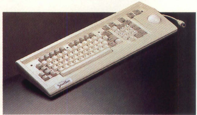
Figure 4: Trackball and keyboard are included in one enclosure in the programmable Wico Smartboard; it can be used either as a Dvorak or standard Qwerty device.
