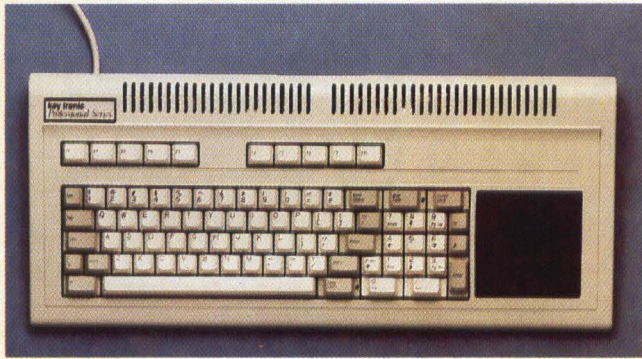
Figure 5: This Keytronics subsystem with touch pad and keyboard also has ports for other input devices.
