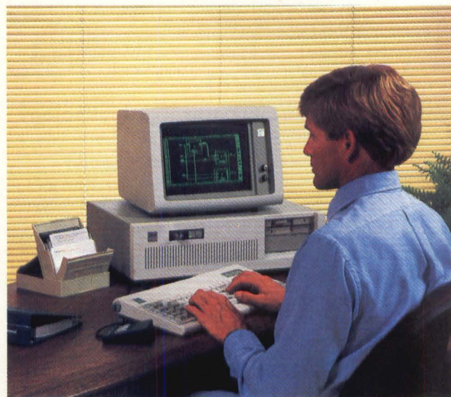
Figure 5: Futurenet's Dash-1 and Dash-2 can be configured on the IBM PC XT or AT. In addition, these systems can be equipped with the Dash Cadat, a 32016 co-processor board with 1 Mbyte of RAM, providing designers with simulation and timing verification.
