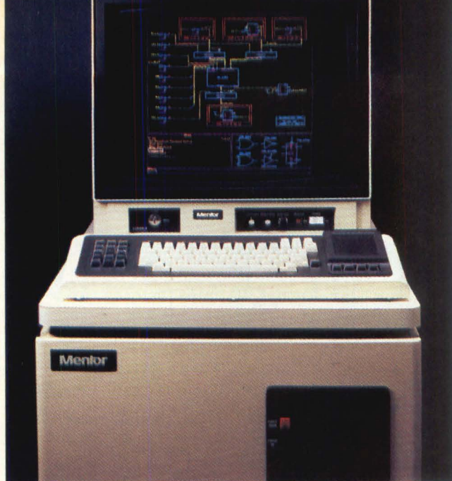
Figure 4: Mentor's high-end workstation, based on the Apollo DN660, offers very good graphics and provides execution speeds just below that of a VAX 11/780. Like Daisy and Valid, Mentor offers a hardware accelerator that significantly speeds logic simulation.
