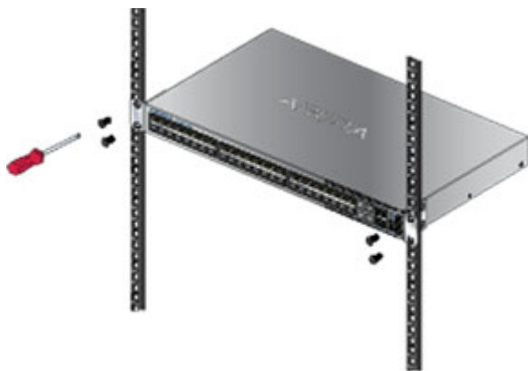
Figure 3-3: Inserting the Switch into the Rack
