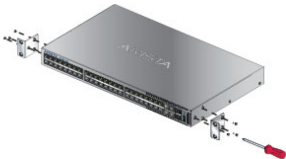
Figure 3-2: Bracket Mount Attachment to Switch
