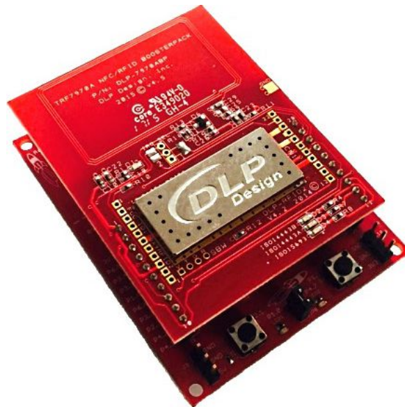
Figure 13. MSP430F5529 LaunchPad Development Kit and DLP-7970ABP BoosterPack Plug-in Module
