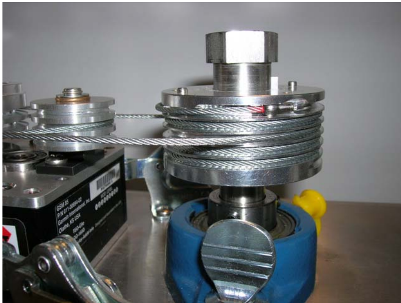
Figure 3-21. Cable wrapped and inserted in upper slot of fixture capstan
