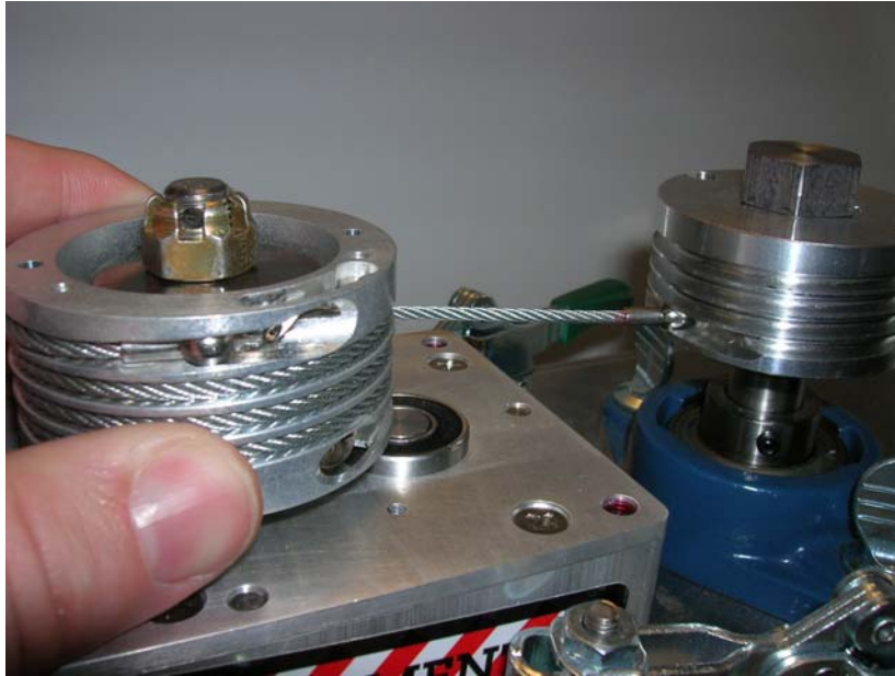
Figure 3-12. Cable inserted in bottom slot of fixture capstan
