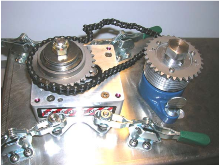
Figure 3-24. Sprocket capstan installed on fixture
