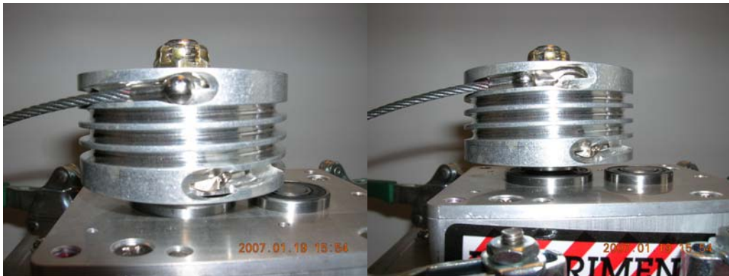
Figure 3-10. Inserting 3/32 cable in the unit capstan.
