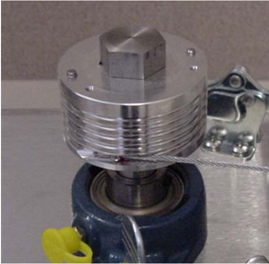
Figure 3-6. Cable Placement (fixture capstan)
