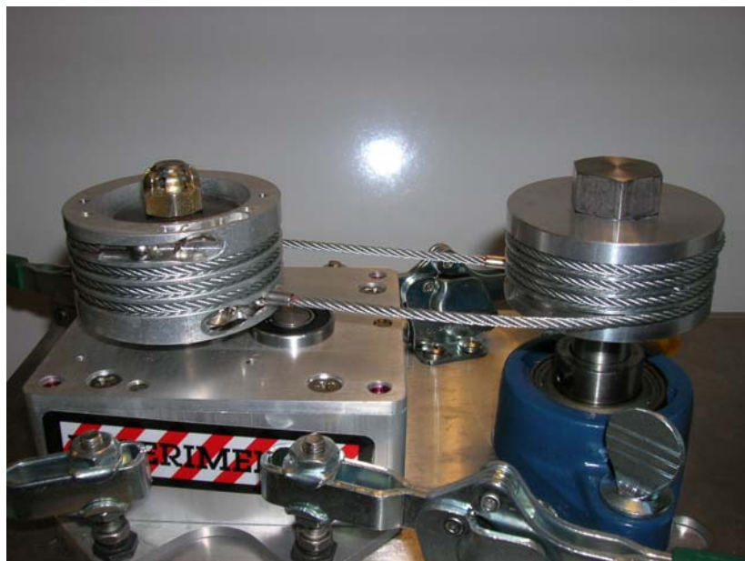
Figure 3-14. Cable wrapped around test fixture capstan, remaining end installed in unit capstan bottom slot
