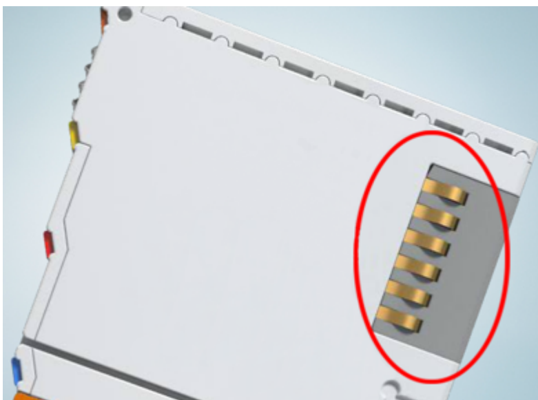
Fig. 29: Spring contacts of the Beckhoff I/O components
