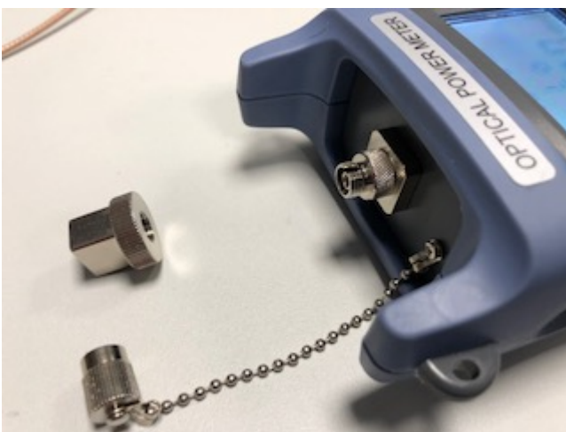
Fig. 51: OPM with FC adapter screwed on
