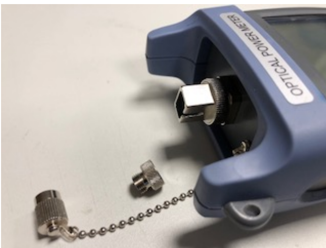
Fig. 52: OPM with SC adapter screwed on
