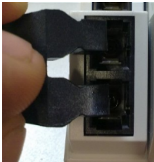
Figure: Blind plugs in unused sockets
