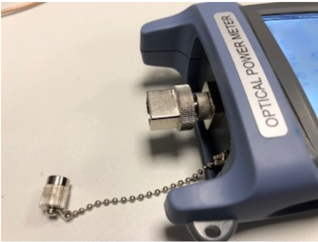
Fig. 53: OPM with FC and SC adapter screwed on - WRONG
