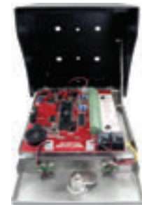
Hinged faceplate allows for easy access
