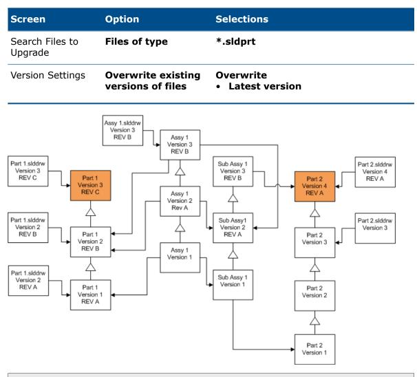
By default, part drawings are not upgraded. However, because drawings are parents to parts, a Broken reference warning screen lets you select to upgrade the drawings that reference the parts that are being upgraded.
