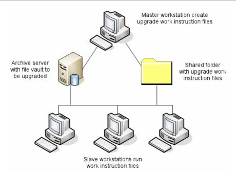
The work instruction files contain tree structures that reflect the parent-child relationships of the SOLIDWORKS files. Both master and slave workstations can run additional work instruction files after they finish processing the first one. Although parts and subassemblies can be shared by other assemblies, each file is only upgraded once.
