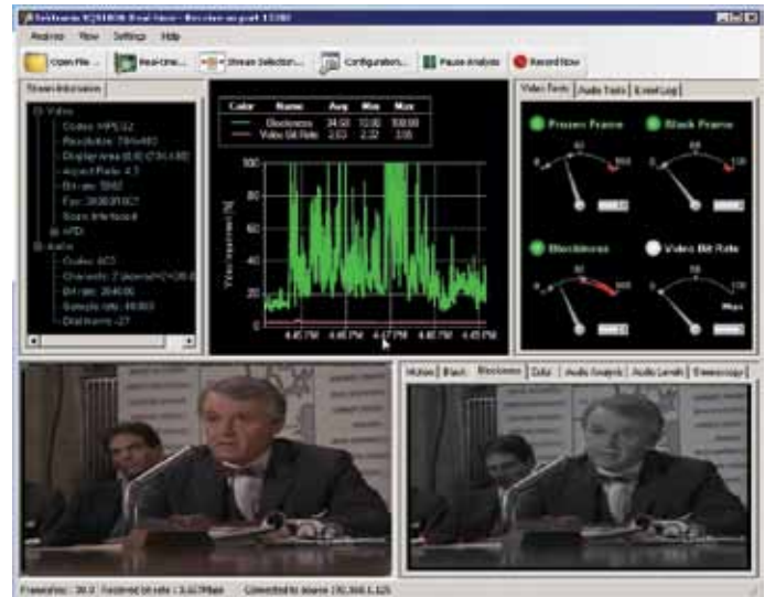
Figure 3.11. Transcoded content with significantly higher blockiness (green plot) over the same timeframe.
