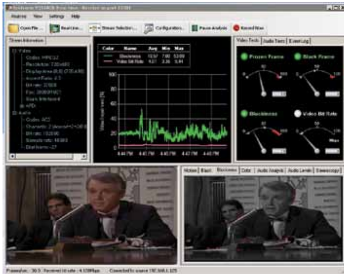
Figure 3.10. Low blockiness from satellite distribution feed.
