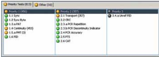
Figure 3.5. TR 101 290 table tabulating several corrupt TS packets as well as lost or missing packets.
