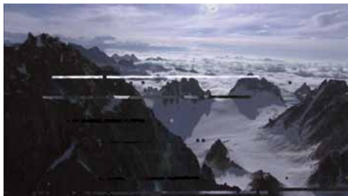
Figure 3.15. Significant loss of RF or IP packets cause blockiness and slice errors.
