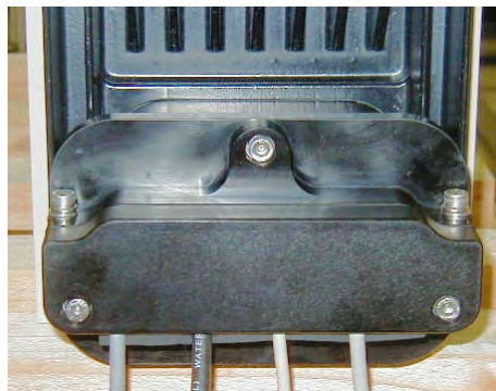
Figure 9-7. Splash Guard Installed
