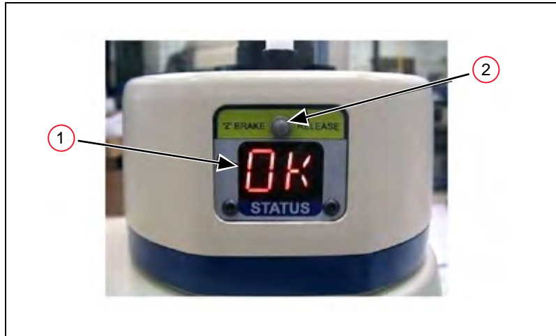
Figure 5-2. (1) Status Panel for Displaying Fault Codes, (2) Z Brake Release Button - Upright Model Shown.
