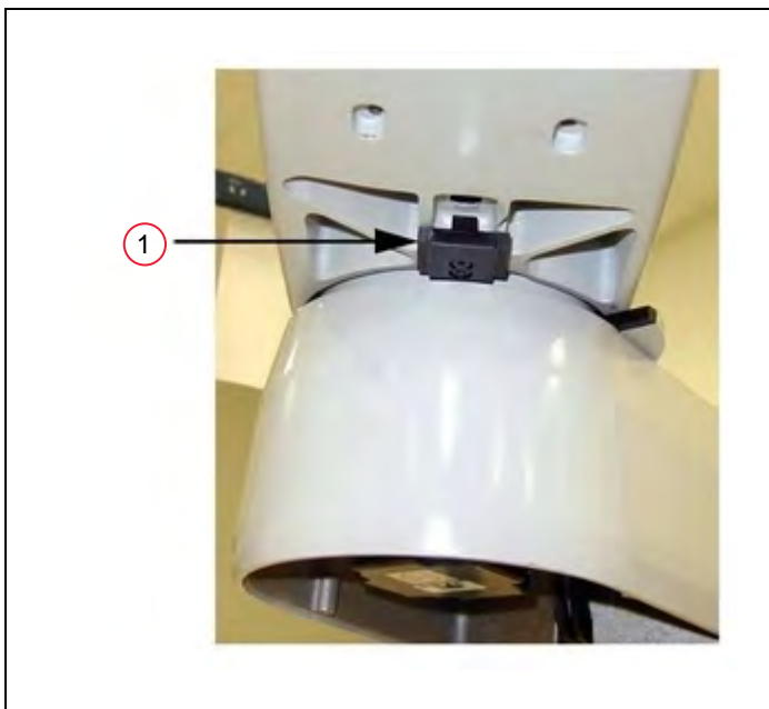
Figure 7-23. (1) Fixed Hardstop Block for Joint 2
