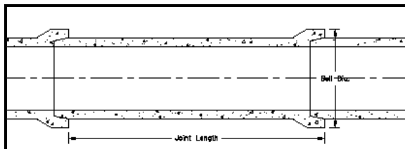
Typical Concrete Pipe Configuration
