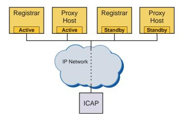
In this scenario, one redundant server pool is assigned to the primary Registrar and another redundant server pool is assigned to the primary Proxy during system provisioning.
