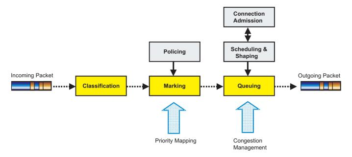
The individual functions are used to accomplish specific tasks for QoS.
