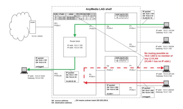
The following figure shows a routing between two subscribers connected to the  $AnyMedia^{\text{(B)}}$  Access System. Again, the VLAN ID is being changed by the router block.
