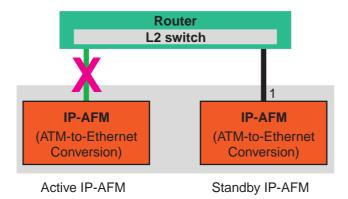
This deployment is used when the network router/L2 switch does not support the RSTP protocol.
