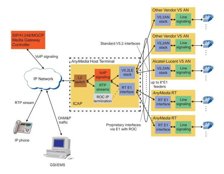
The standard V5.2 aggregation and remote terminal (RT) aggregation via the proprietary remote terminal signaling and control interface are supported within one image (mixed aggregation-share of the E1 feeder) and are different in the following aspects:
