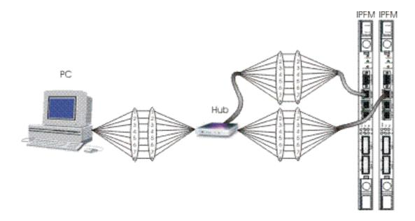
When controller packs (for example IPFMs or IP-AFMs) are used in duplex mode on a single shelf, the LAN interfaces are joined at a hub or by a special Y-assembly. In either case, both controller packs use the same IP address.
