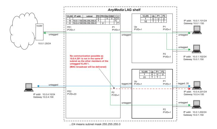
The next figure shows L3 VLANs, where source IP address and destination IP address are not located in the same subnet. Therefore the routing capability of the packs in the *AnyMedia*® Access System is required. Shown is a possible route (note that the VLAN ID is being changed by the router block) and an example where no routing is possible because for VLAN ID 1 no IP address is specified.
