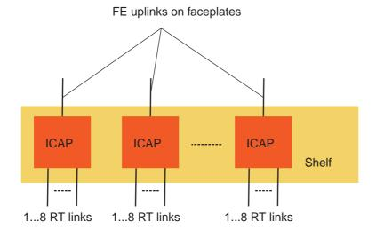
In contrast to the IPFM controlled mode, the management system has to treat each IP AP (or a pair of ICAPs in duplex mode) as a completely independent system.
