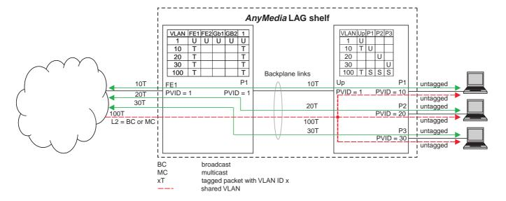
The next figure shows how packets are handled in the AnyMedia® Access System in an untagged shared VLAN in the network.
