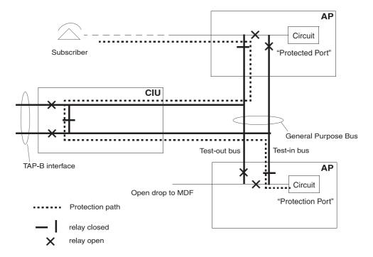
The 1:N protection for application pack ports supports only manual protection switching, that is, on operator demand. It is solely on operators discretion whether to switch a protection for a specific port, probably based on test results from former metallic line tests, circuit tests or due to subscriber complaints.
