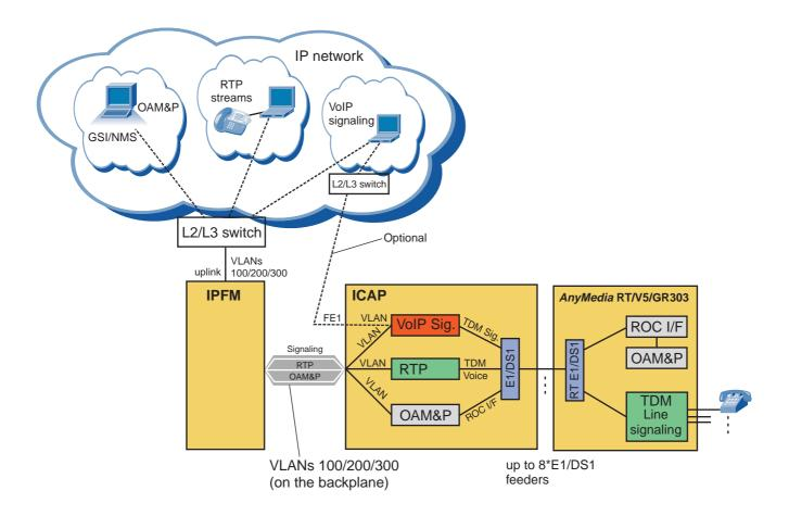
The diagram below shows the stand-alone mode (The ICAP is not controlled by the IPFM).
