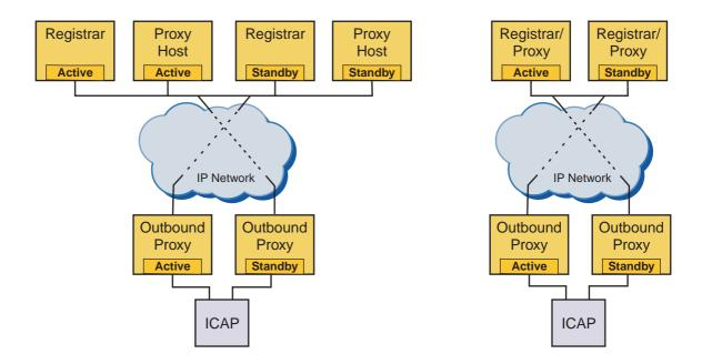
The Outbound Proxy has to support a redundancy mechanism for the Registrar and/or Proxy host in this scenario. The ICAP does not provide a redundancy for the Registrar and/or Proxy host but only for the Outbound Proxy host.
