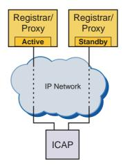
In this scenario, one redundant Registrar/Proxy server pool is assigned to the ICAP during system provisioning.
