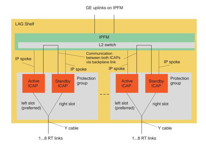
The next figure shows two ICAP protection groups in stand-alone mode. In this example the left ICAP in each protection group is in active mode.
