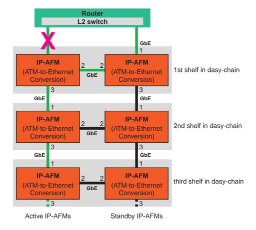
Link failures and pack problems are handled by the RSTP protocol machines running on each of the participating IP-AFMs. No special fault handling mechanism is required to protect the paths between the packs and the network.
