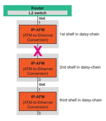
In simplex deployments the RSTP protocol machine is turned off since there are no alternative paths to search for in case of failures and RSTP operation would block traffic from daisy-chained shelves connected to an IP-AFM recovering from a pack failure.
