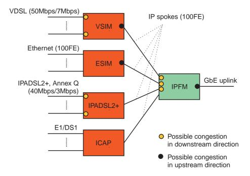
The next figure shows possible congestion points in the system using an FE uplink.
