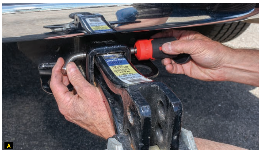
A) Bolt's \frac{5}{8} -inch Receiver Lock keeps the 2-inch receiver hitch in place and secure. It also prevents the unhitched trailer from being stolen.
