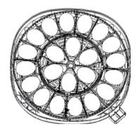
After setting the eggs, conduct a turning test to check if each egg is sitting correctly and can turn smoothly. Conduct the test run by pressing the "+" and "-" buttons at the same time. To make observation easier, the sides of the eggs can be marked with a pencil mark "X".
