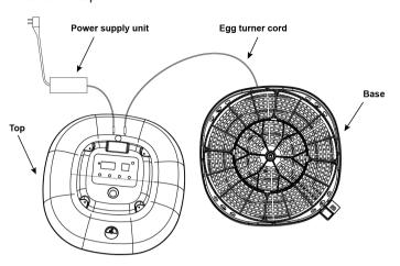
d) Place the top onto the incubator base, ensuring the clear window is completely closed. It's important to align the two notches on the bottom of the clear window with the two sockets on the base.
