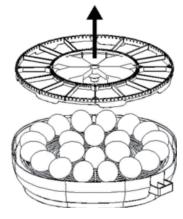
Remove the red plug from water pot "B", fill both water pot "A" and "B". and adjust the air vent knob to achieve a higher humidity around 70%.
