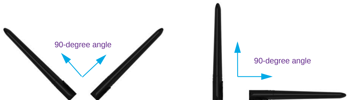
Figure 4. Recommended antenna angle
