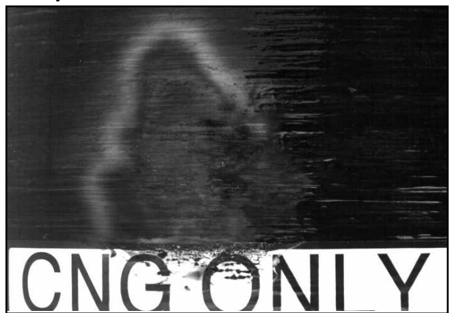
Figure 6-17 Level 3 Heat Damage Discoloration and Resin Burnout (Condemn)
