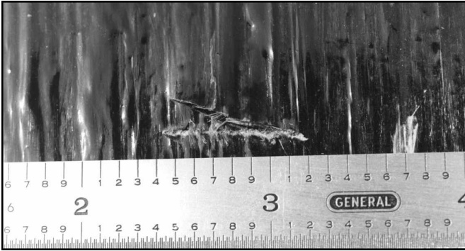
Figure 6-14 Level 2b Loose Fiber From Gouge Damage
