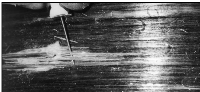
Figure 6-13 Level 2a Loose Fiber Damage (Customer Rework)
