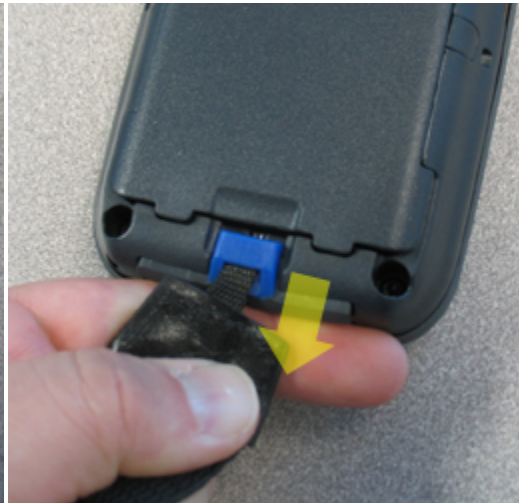
Pull on Strap to Release Battery
