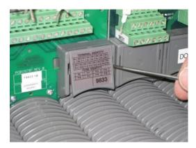
2. Find the **open fuse** and remove it. Rockwell Automation recommends the use of catalog number T9908 fuse removal tool or equivalent long nose pliers. Pull the fuse slowly straight out to prevent damage to the fuse holder.
