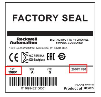
For AADvance product still in its original carton, the product identification information will be on the product carton label. The catalog number will be in the "CAT" field and the date of manufacture will be on the right side under the dividing line and will be of the format YYYY/MM/DD where YYYY is the year, MM is the month code, and DD is the day of the month.
