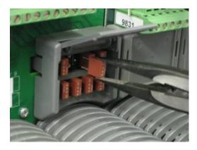
3. Insert the **new fuse**. Push the fuse straight into the fuse holder to avoid damage.
