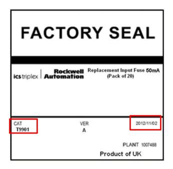
AADvance T9901 replacement fuse 20 pack kits may be used for both 1715 Redundant I/O and AADvance input termination assemblies. Individual fuses are not marked with date information. The product catalog number is located on the shipping bag label in the CAT field. The manufacturing date is located on the right side below the dividing line and will be of the format YYYY/MM/DD where YYYY is the year, MM is the month code, and DD is the day of the month.
