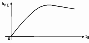
FIGURE 1.10 EMITTER-CURRENT DEPENDENCE OF h_{FE} IN A SILICON TRANSISTOR
