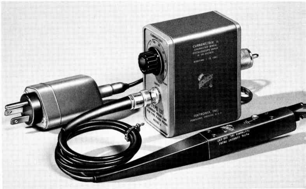
FIGURE 20.2 CURRENT PROBE AND AMPLIFIER
