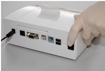
Picture 9: Powering up
