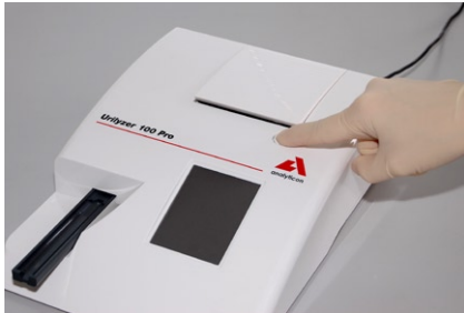
Opening the printer cover
