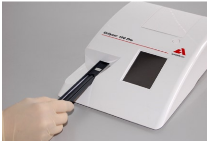
Loading test strip tray
