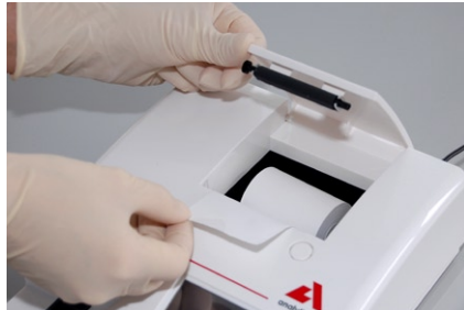
Loading the printer paper
