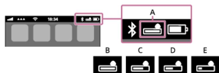
**A:** Remaining battery charge of the headset
