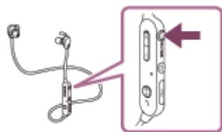
Press the NC/AMB button repeatedly. A voice guidance informs you that the setting has switched. Each time you press the button, the function is switched as follows.
