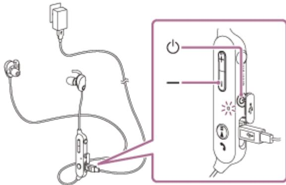
If the headset does not operate correctly even after resetting, initialize the headset to restore factory settings.
