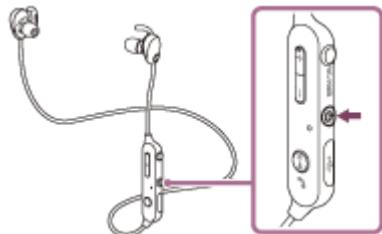
Make sure that the indicator flashes blue and red alternately after you release the button. You will hear a voice guidance "BLUETOOTH pairing".
