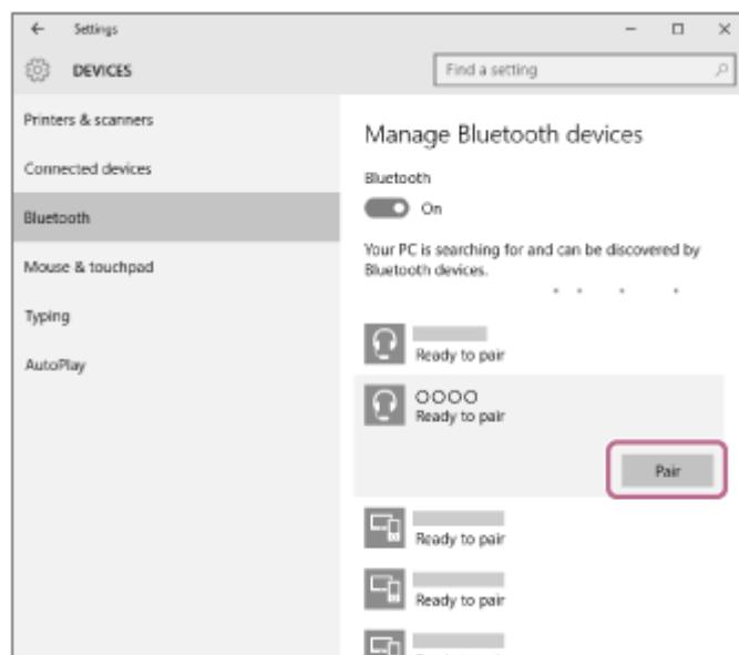
If passkey (\*) input is required on the display of the computer, input “0000.”
