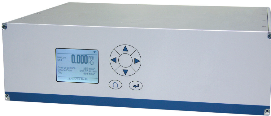
FIG. 2. New CLD instruments a offer a low \text{NO}_x detection limit of 0 ppm–10 ppm.
