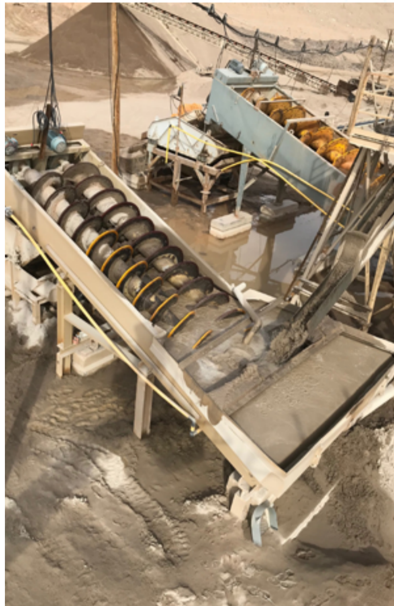
Figure 3: Material Washer Wet process auger screws wash the rocks or sand with water.
