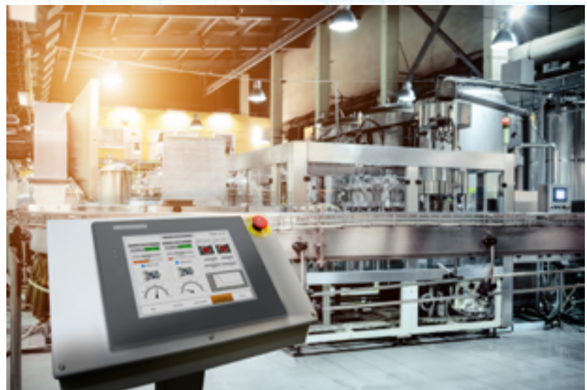
Figure 3: C-more. When traditional VPNs are used, a local HMI, such as this AutomationDirect C-more panel, is often part of the solution.
