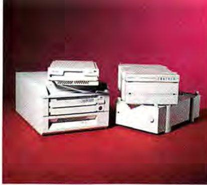
figure 4 / Drives with a difference. The MegaDrive Mercury 240 (left) lets you remove the hard drive from the base and lock it away for safekeeping. The Mirror SmartStack system (right) forms a neat storage tower as you plug drive modules in to the base.
