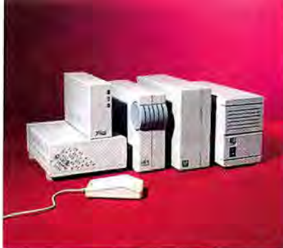
figure 2 / Smallest of the small. Of the totable candidates, only the Liberty 50 Series drive (upper left), with its battery or AC operation, is truly portable.
