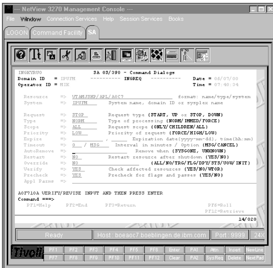
Figure 142. NetView Console with INGREQ Panel
