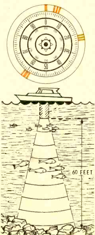
Dial shown indicating fish at two levels, plus bottom at 60'.
