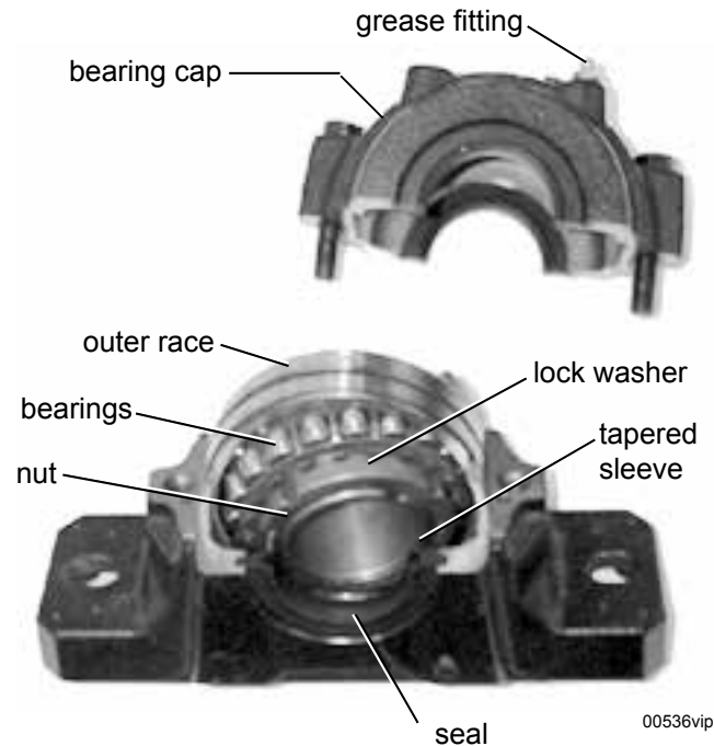
FIGURE 32 - SPLIT BEARING
