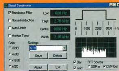
The DSP applet provided with the WR3000 allows continuous control of audio bandwidth and other signal conditioning functions
