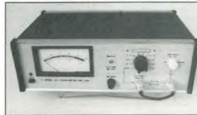
RF Power Meter Model 2081. to 500MHz. 100W. 50ohms. 7 ranges
