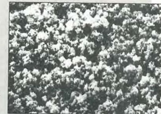
Fig. 14. Large magnification electron microscope view of the surface of a very high 'gain', low-voltage anode foil. Etching and forming methods are optimised for low voltage capacitor use.
