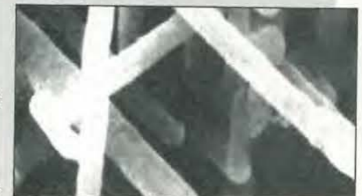
Fig. 15. Very large magnification electron microscope sectional view of low surface gain, very high voltage etched foil. Shows extensive large diameter tunnels able to accept thicker oxide growth needed for high forming voltages. Only the oxide tunnels are seen, the metal having been dissolved away to permit this sectional view.
