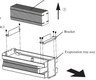
® Remove 4 screws that attach to the lower evaporation tray and lower moisture wicking plate. Then remove the tray assembly and the moisture wicking plate.
