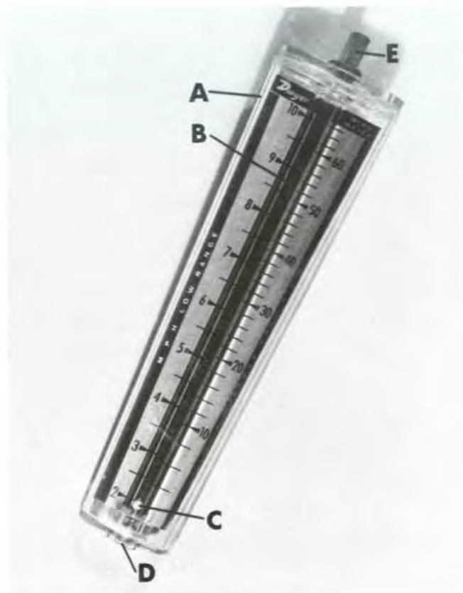
Figure 31.10 —Dwyer hand-held wind meter: A, outer shell; B, inner tube; C, indicator ball; D, bottom plug; E, top stem.
