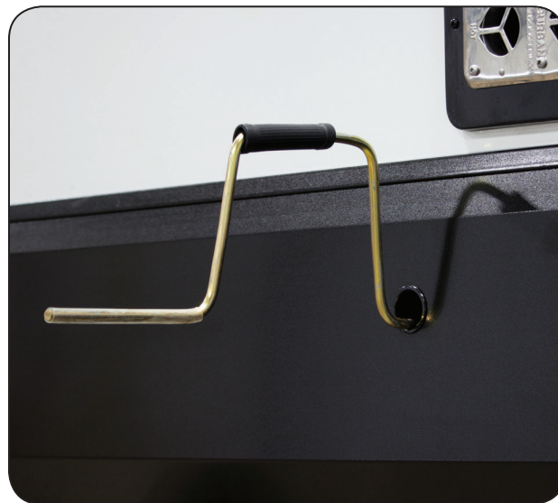
Slideout Override Access Hole & Crank Handle Extension
