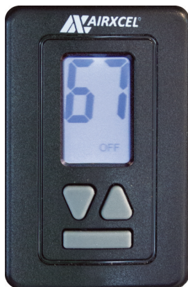
The Digital Thermostat is wall-mounted inside the RV
