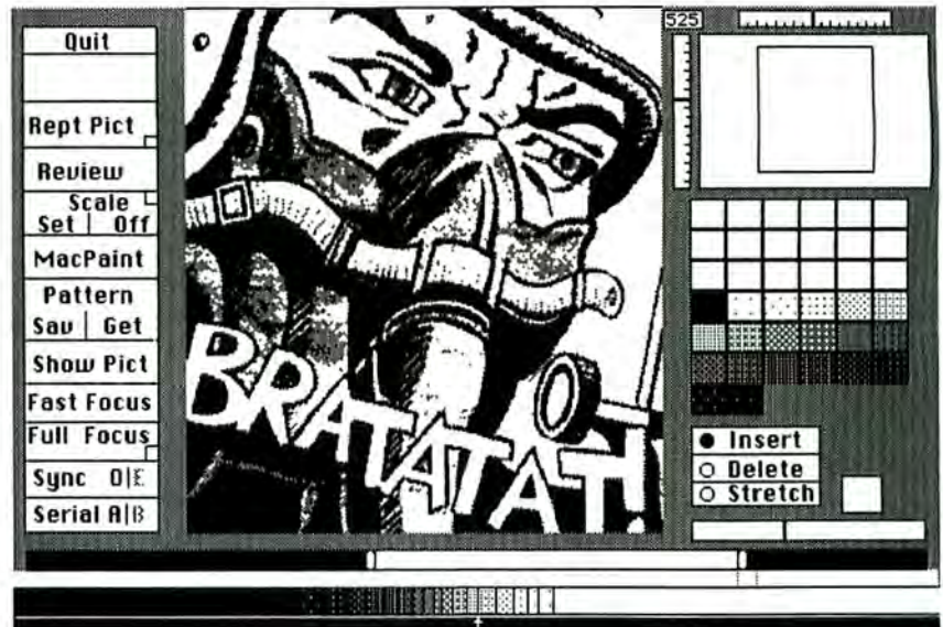
Figure 3 The Magic control panel lets you review previously digitized images, focus the image, change and edit patterns, and adjust contrast and brightness. The box and rulers in the panel's upper-right corner are the pan control. You can select patterns from the palette and place them on the pattern bar; the thickest horizontal bar at the bottom of the screen.
