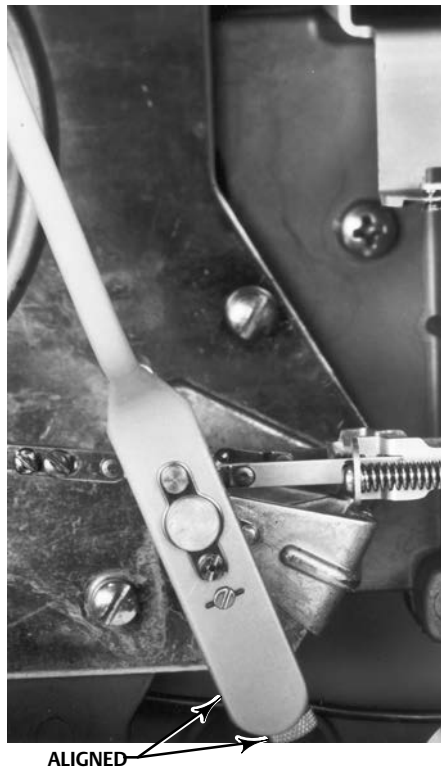
Figure 5-6. Process Indicator Alignment
