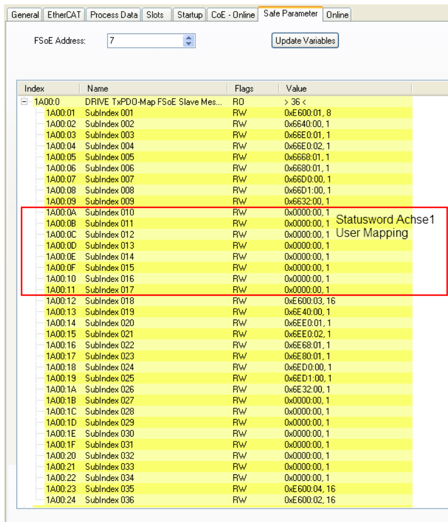
Fig. 18: Status word user mapping for axis 1
