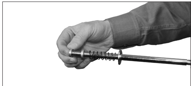
Fig. D: Remove 2 nuts and spring from threaded rod. Leave the washer on the rod.
