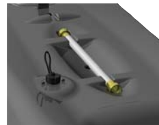
Self-storing water hose for easy tank cleaning.
