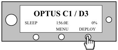
• Press **DEPLOY** will deploy system. Then antenna will lock onto target satellite automatically.
