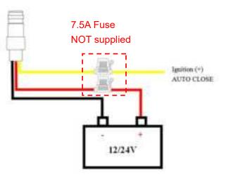
Red: Positive of battery(VBAT+)Black: Cathode of battery(VBAT-)Yellow: Ignition(+)
