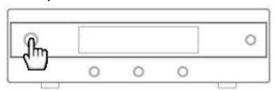
Turn On Power The antenna system will retract to shut down position and enter into Sleep Mode. The power consumption is very low.
