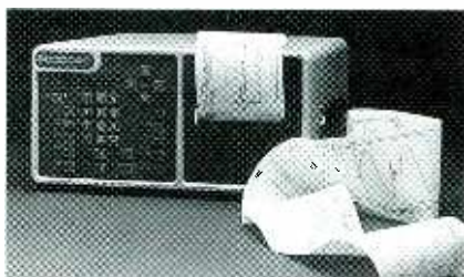
FIG. 4—THE BMI 4800 POWERSCOPE. While similar to the BMI 2400 in physical appearance, it has considerably more processing power, with up to four main and eight probe channels.
