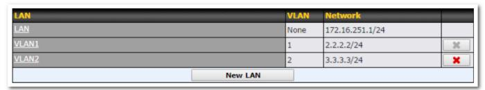
This represents the LAN interfaces that are active on your router (including VLAN). A grey "X" means that the VLAN is used in other settings and cannot be deleted. You can find which settings are using the VLAN by hovering over the grey "X".
