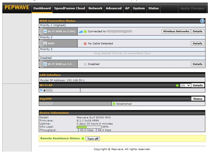
The **Dashboard** shows current WAN, LAN, and Wi-Fi AP statuses. Here, you can change WAN connection priority and switch on/off the Wi-Fi AP.
