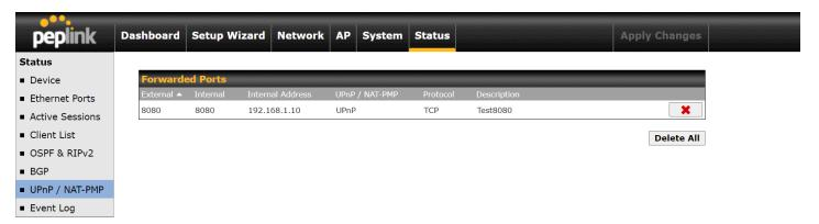
In the example above, the UPnP device is running. When the UPnP device is disconnected, the router will suspend the service and incoming traffic will be dropped (without error/notification message). The UPnP rule will remain for an interval after the UPnP device is disconnected before being removed.
