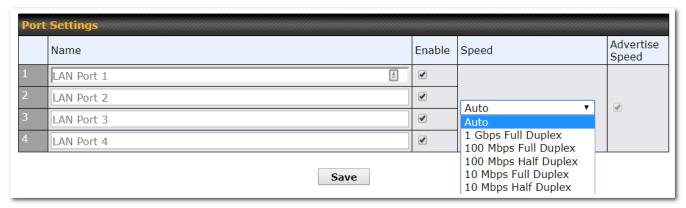
On this screen, you can enable specific ports, name the LAN ports, as well as determine the speed of the LAN ports.
