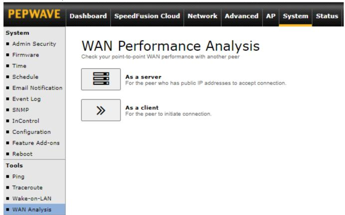
The default port is 6000 and can be changed if required. The IP address of the WAN interface will be shown in the **WAN Connection Status** section.
