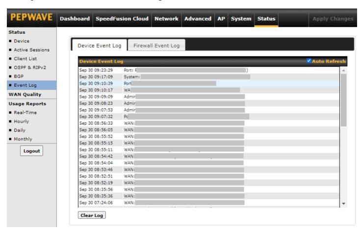
The log section displays a list of events that has taken place on the Pepwave router. Check **Auto Refresh** to refresh log entries automatically. Click the **Clear Log** button to clear the log.
