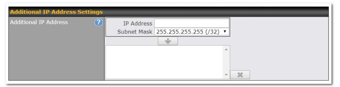
Enter the subnet IP Address and Subnet Mask, press the down arrow button, and the list will be populated by the IP addresses of the specified subnet. You should delete the WAN connection's primary IP address and the gateway address from the list by pressing the *Delete* button after selecting them in the list. These additional IP addresses can be assigned to a device on the LAN using NAT Mappings
