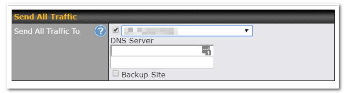
You can (optionally) specify a DNS server to resolve incoming DNS requests. Click the checkbox next to **Backup Site** to designate a backup SpeedFusion profile that will take over should the main PepVPN connection fail.
