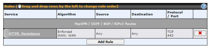
The bottom-most rule HTPS\_Peristence is **Default**. This rule manages the device's default manner of controlling outbound traffic for all connections that do not match any of the rules above it. To rearrange the priority of outbound rules, drag and drop them into the desired sequence.
