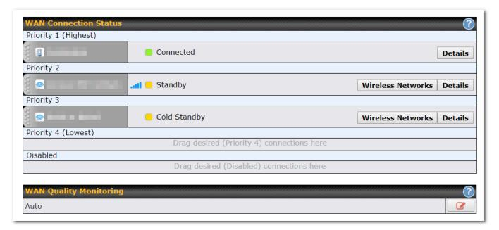
To disable a particular WAN connection, drag on the appropriate WAN by holding the left mouse button, move it the **Disabled** row, and drop it by releasing the mouse button.
