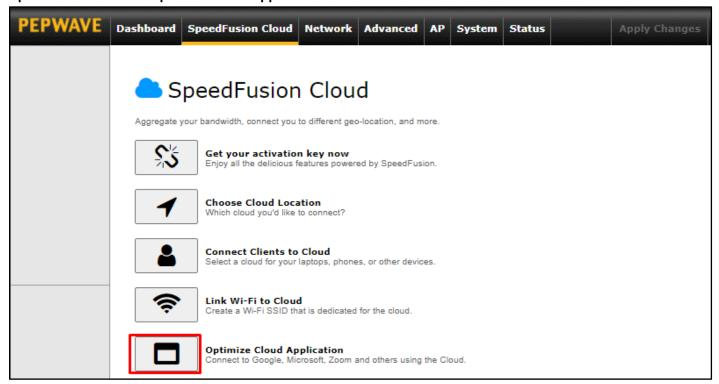
Select a Cloud application to route through SpeedFusion Cloud from the drop down list > Click > Save > Apply Changes. Click the to remove a selected Cloud application to route through SpeedFusion Cloud.
