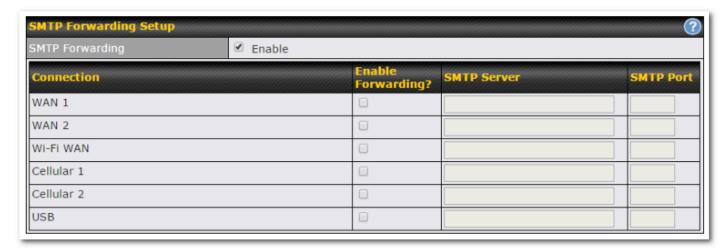
To enable the feature, select **Enable** under **SMTP Forwarding Setup**. Check **Enable Forwarding** for the WAN connection(s) that needs forwarding. Under **SMTP Server**, enter the ISP's email server hostname or IP address. Under **SMTP Port**, enter the TCP port number for each WAN.
