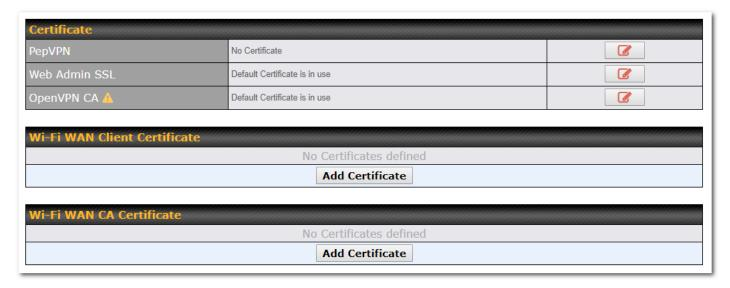
This section allows you to assign certificates for the local VPN, OpenVPN, Captive Portal, Mediafast, Contenthub, Wi-Fi WAN (Client and CA) and web admin SSL for extra security.
