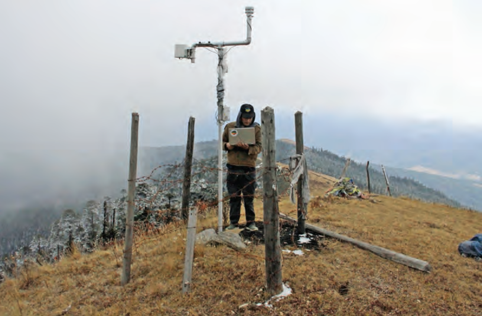
Downloading data from a high-altitude automatic weather station in the UWICE research preserve, Bumthang, Bhutan. © WWF Bhutan
